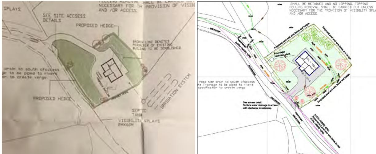
Figs 3 & 4: Site layout including access previously approved under planning application M/2008/0556/F and site layout including access currently sought, respectively.
