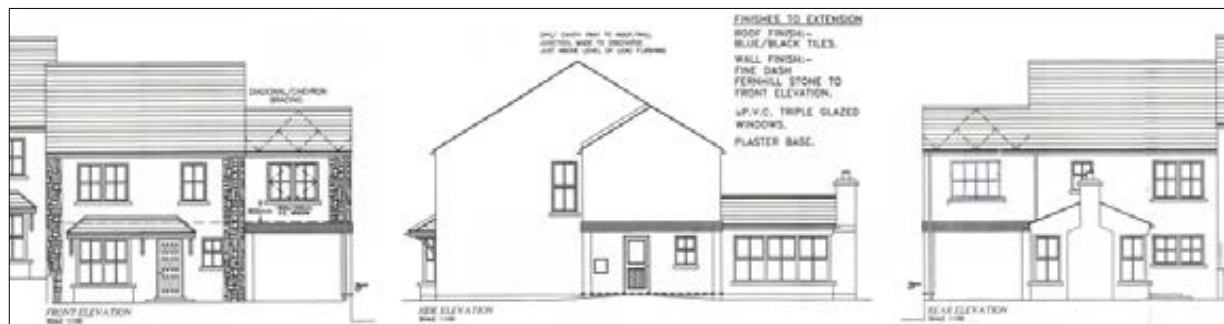
Fig 3: Proposed front, side and rear elevation of proposed extension, respectively.
