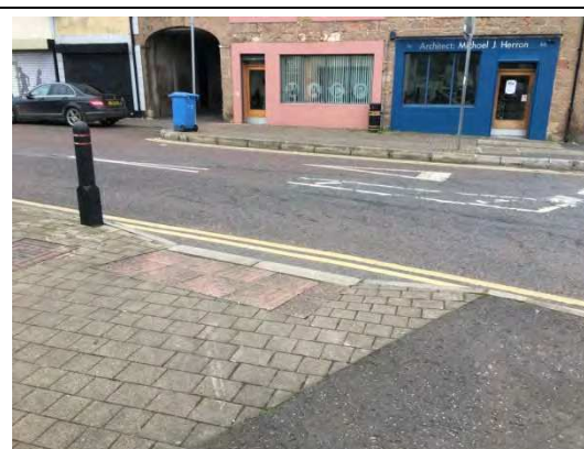
Main St - Pedestrian crossing with no complimentary dropped kerb on opposite side of the road which presents a safety issue
