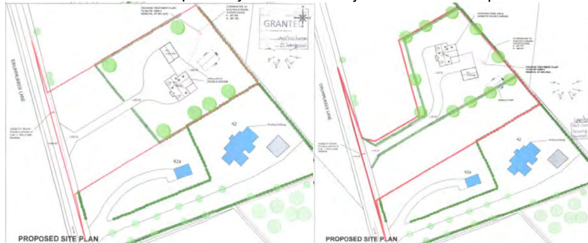
Figs 5 & 6: Site layout including location of dwelling and garage previously approved; and new site layout including relocation of the dwelling and garage sought, respectively.
