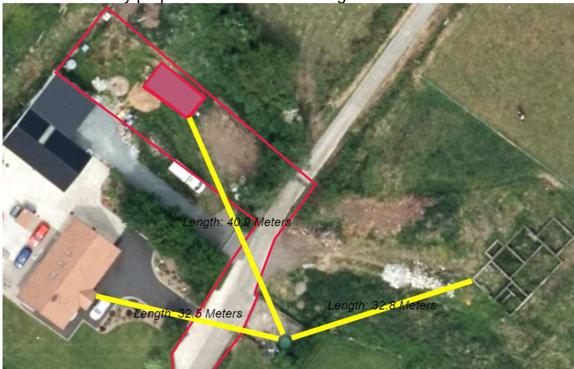
Fig 7: Showing WwTw's in relation to proposed dwelling (red box on site); and two houses located at a closer distance to the existing tank, one of which consists
