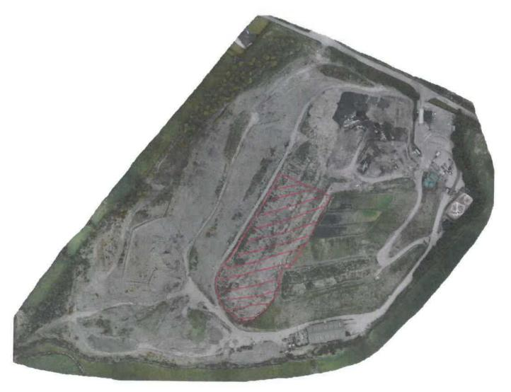
The works will mainly consist of the installation of a composite capping system as well as the installation of a bund for stability and drainage. The capping system has been designed to meet the requirements of the Landfill Regulations (Northern Ireland) 2003.
