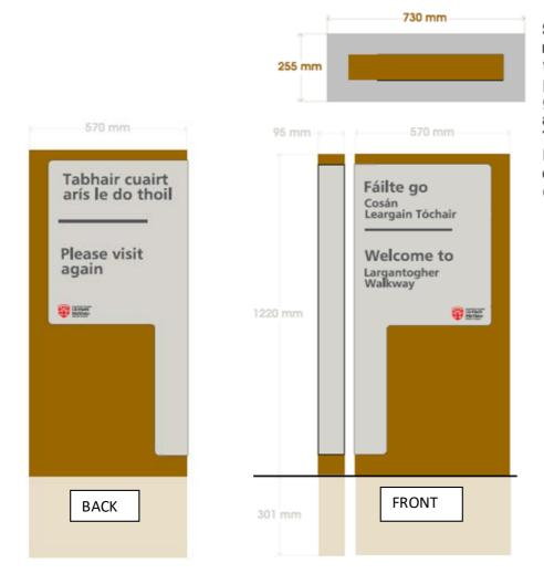
Signage comprised of 95mm2 'brown' recycled plastic posts securely fixed together with hidden fixings, the posts will be concreted into the ground with a 255mm\*730mm plinth around it level with the ground. The faceplate is to be made of brushed silver composite material with text directly applied.
